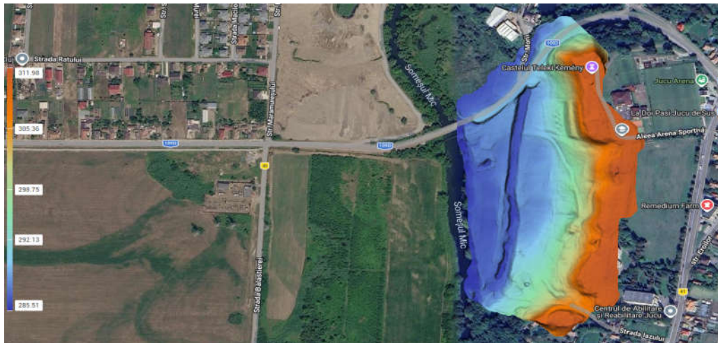
Figure 5. Digital Elevation Model (DEM) of the study area derived from the LiDAR ground point classification (LiDAR360). The morphological transition from the castle promontory slope (northwest) to the Someșul Mic floodplain (east) is clearly.
